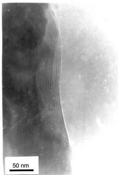
Fig. 4 TEM image of a \text{TiO}_2\text{-C}_{16}\text{TABr} film prepared at 50^\circ\text{C} in air.
